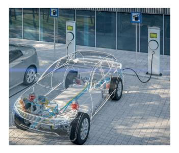
DC/DC CONVERTER: This device converts higher-voltage DC power from the traction battery pack to the lower-voltage DC power needed to run **your vehicle's** accessories and recharge the auxiliary battery.
