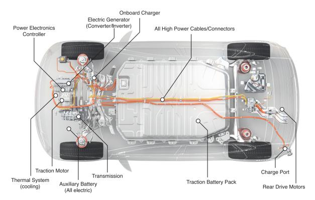
**ELECTRIC TRACTION MOTOR:** Using power from the traction battery pack, this motor drives the vehicle's wheels. Some vehicles use motor generators that both drive the wheels and charge the battery.
