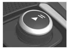
Volume/Play/Stop/Pause Control Rotate to adjust volume, press the centre II⊲ button to play/stop the radio or play/pause media on connected devices. Press and hold the button for 2 seconds to activate screen cleaning mode, see the main owners handbook for further information.
